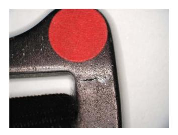
Case study - harness with a fault from new. The harness was used for some time before the fault was found. An initial inspection would most likely have spotted this.
