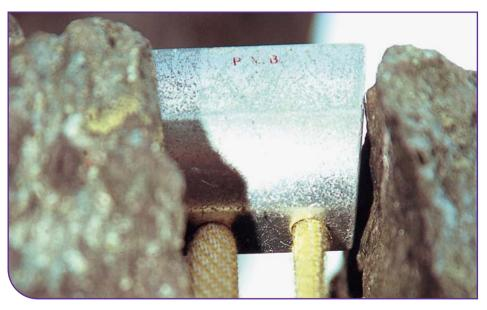
Figure 4.3 An example of poor placement in rock – the nut is not 'seated' with all of its edges in contact with the rock Photo: Alex Messenger
