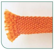
Figure 12.2 Cut, damaged yarn
