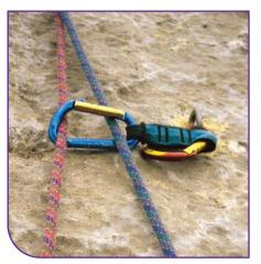
Figure 1.5 Badly-positioned karabiner Photo: George Steele
