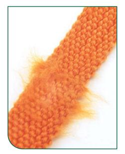
Figure 11.4 Frayed/damaged webbing
