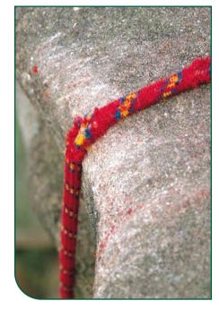
Figure 10.3 Serious damage to a rope in use Photo: BMC Collection
