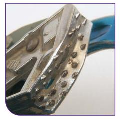
Figure 6.4 Ascender with worn and damaged teeth
